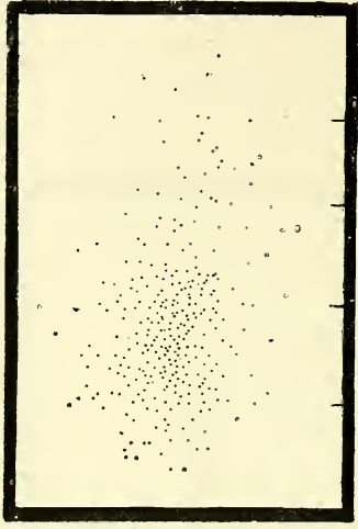
Facsimiles of patterns showing both lateral deviation and stringing of the same pellets.
